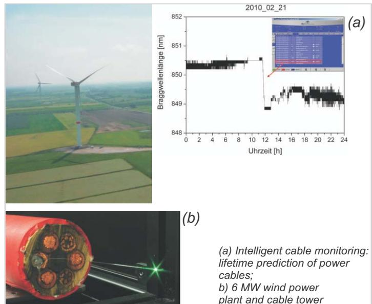
User example of TAMA in a 6 MW wind power plant.
